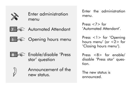
The "Press star' question can be used to check whether the dialling information sent by the caller could be interpreted correctly or not. The application can only react on signals created by digit keys of a touch—tone phone.
